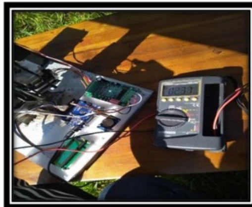
Gambar 4.14 Pengukuran Arus Panel Surya
